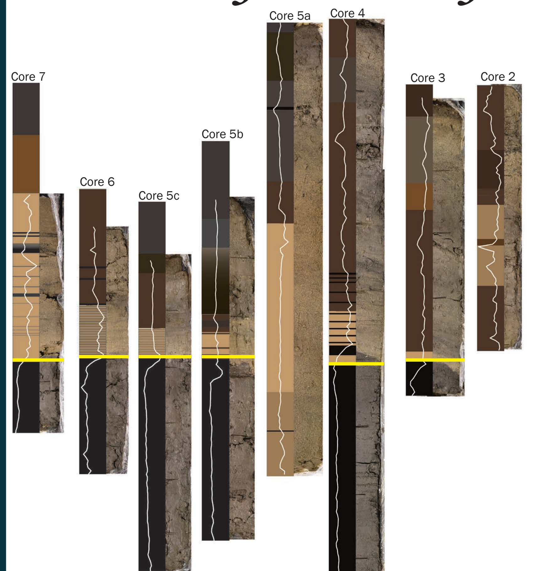
Figure 6. An illustration of the cores collected across the inlet. White lines indicate changes in magnetic susceptibility. Visual analysis of the cores show changes in stratigraphy with depth, as well as the pre-flood to post-flood sediment interface (shown in yellow).
