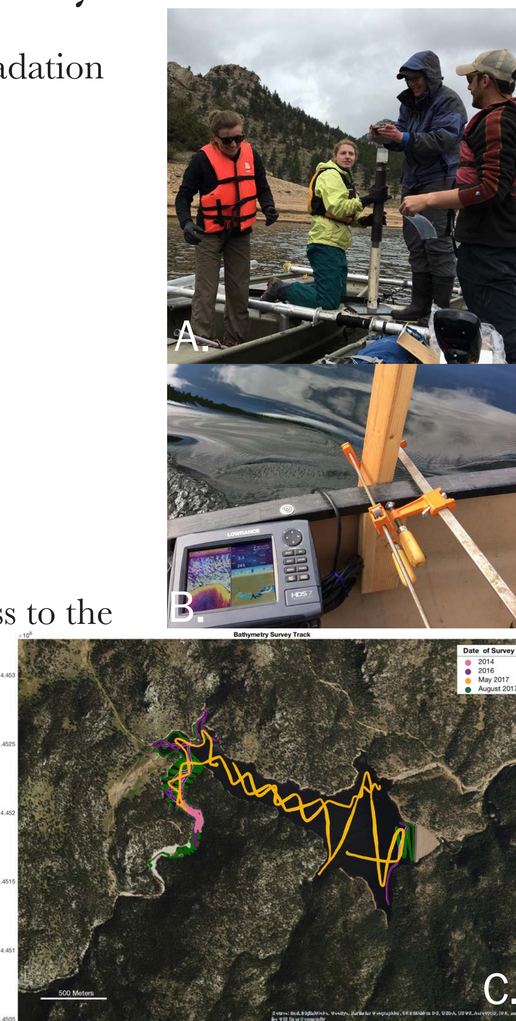
Figure 2. Pictures showing fieldwork including core collection (A) and traces of the bathymetric survey (B). Figure 2c shows the spatial extent of various bathymetric surveys at Ralph Price Reservoir.
