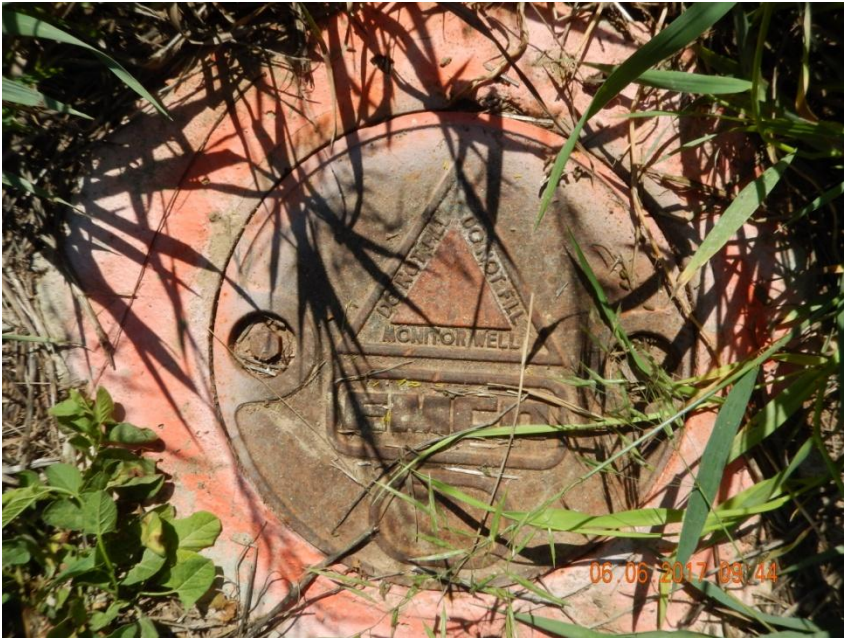
Photo 7. Photo taken of a monitoring well on the well location. It is unclear whether all monitoring wells have been properly plugged.
