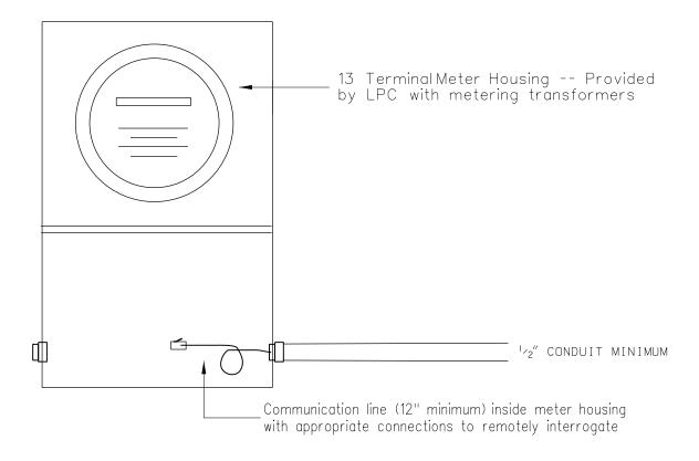
LOAD SURVEY METERING / COMMUNICATION LINE SPECIFICATION
