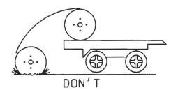
When off loading reels from a truck, lower reels carefully using a hydraulic gate, hoist or fork lift truck. Never drop reels. If reels must be rolled, roll in opposite direction of the cable wraps to keep cable from loosening on the reel.
