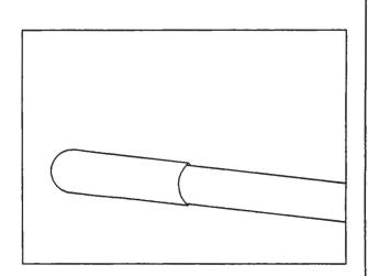
TO PREVENT ENTRANCE OF WATER INTO CABLE, COLD SHRINK SHALL BE INSTALLED ON THE ENDS OF ALL PRIMARY CONDUCTORS
