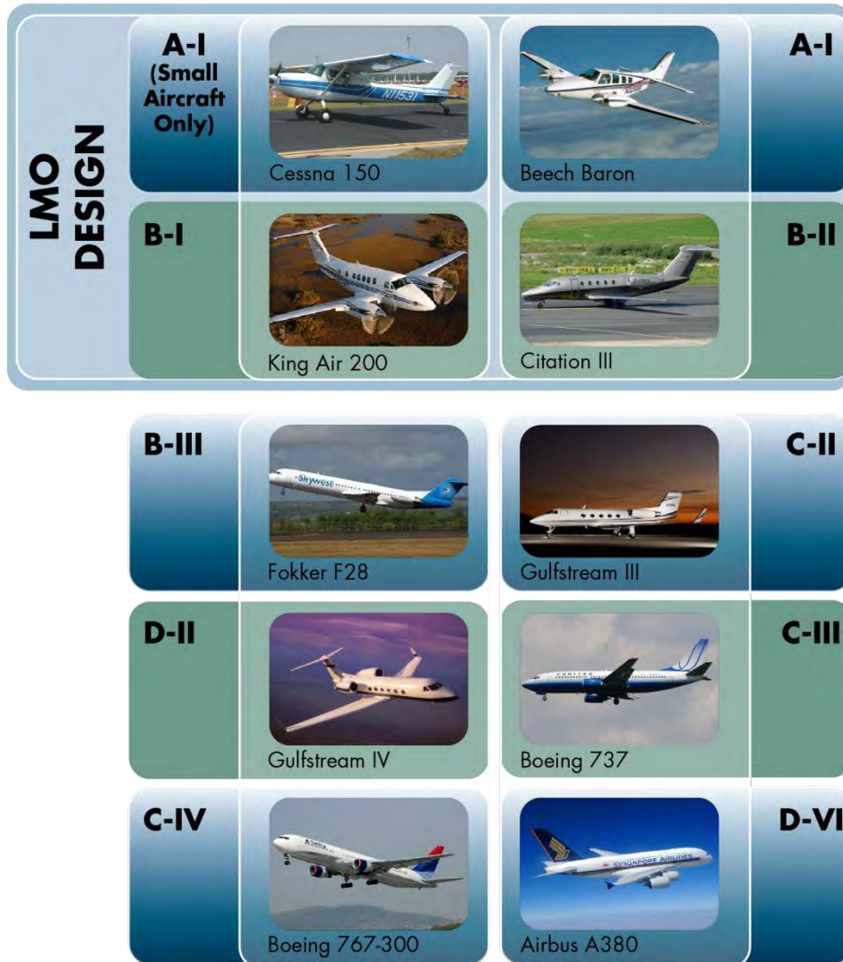
FIGURE 2-1 - ARC AIRCRAFT TYPES AIRPORT REFERENCE CODE (ARC)
