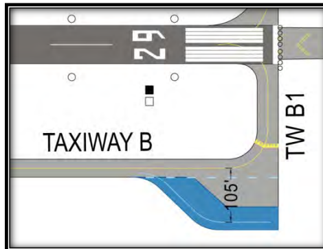
FIGURE 7-8 - HOLDING BAY AT TAXIWAY B1
