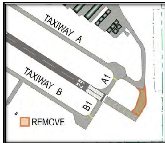
FIGURE 7-4 – REMOVE PAVEMENT ON RUNWAY 29 END
