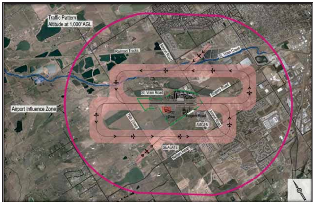
FIGURE 2-6 – RECOMMENDED VOLUNTARY NOISE ABATEMENT PROCEDURES FOR AIRPLANES
