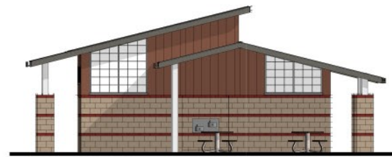
6 BUILDING B RESTROOMS WEST ELEVATION 1/8" = 1'-0"
